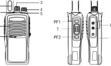
Note: These side buttons PF1, PF2, PF3 can be allocated for certain functionalities. This is can be done with software. The features that can be programmed are listed on backfaces. Each button can be programmed for two features only (Short press 0.5S. Long press 2.5S).
